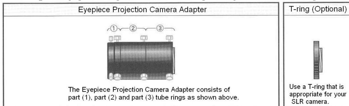
The eyepiece projection camera adapter can be easily coupled onto the 31.7mm visual back of the Vixen flip mirror.
